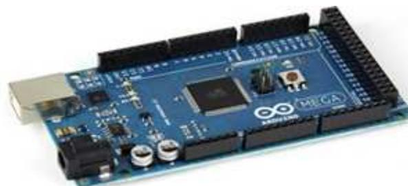
Figura – Arduino Mega
