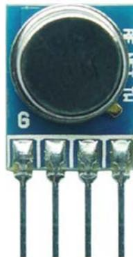
Fig. 2 – Módulo Transmissor RF.
