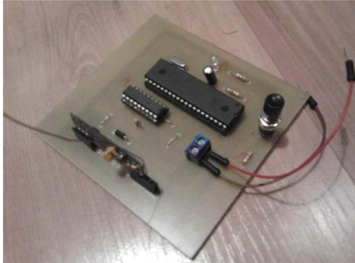
Fig 8. PCI do Receptor RF.
