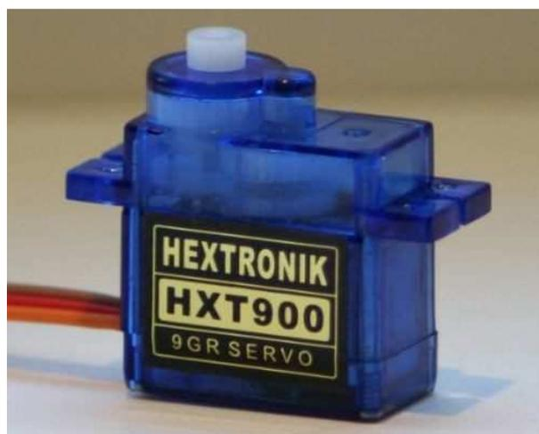
*Micro servo motor Hextronik HXT900, 09 g – torque: 1,6Kg.*
